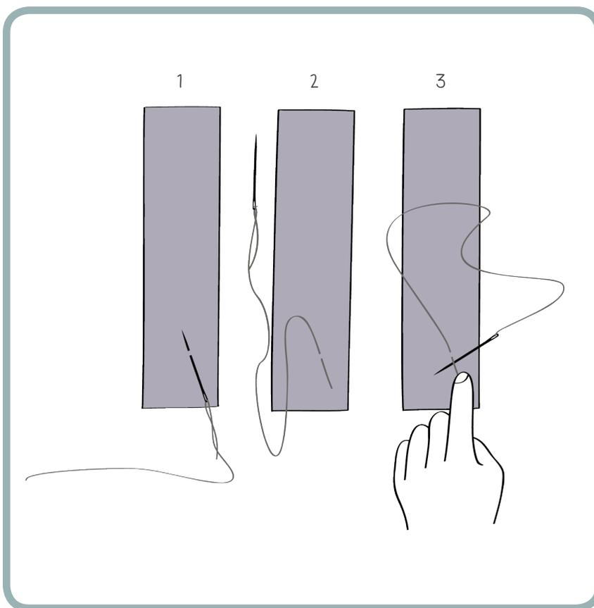
1. On the underside of your fabric, right underneath one of the (+) tabs on your battery holder, sew through a small piece of fabric with your needle. Note: Don't sew through the (+) tab itself, just through the fabric.
