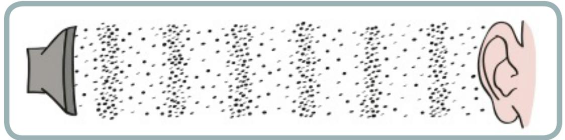
Inside the LilyPad speaker, there is a material that moves in response to electricity. When this material moves, it creates air vibrations and sound.
