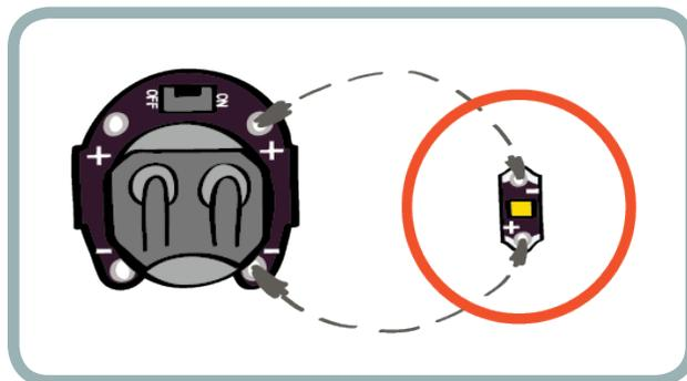
4. Check that the loops around each (+) and (-) tab on the battery holder and LED are snug. If your thread isn't touching one of the (+) or (-) tabs, you'll have a break in your circuit and no electricity will flow.
