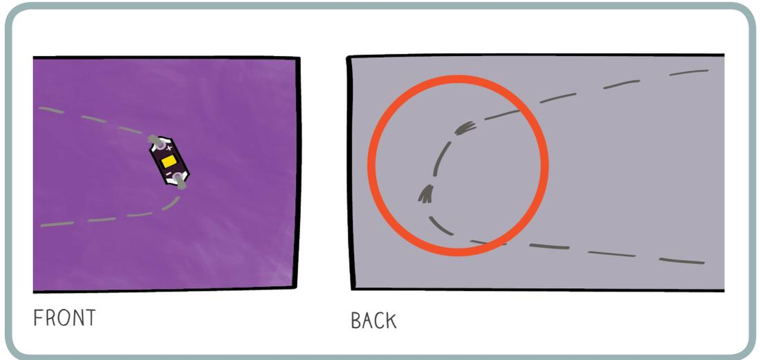
3. Make sure that you've sewn the (+) tab of the battery to the (+) tab of the LED and the (-) tab of the battery to the (-) tab of the LED. If the LED is reversed, it will not turn on. You should take it out and sew it back on in the correct orientation.
