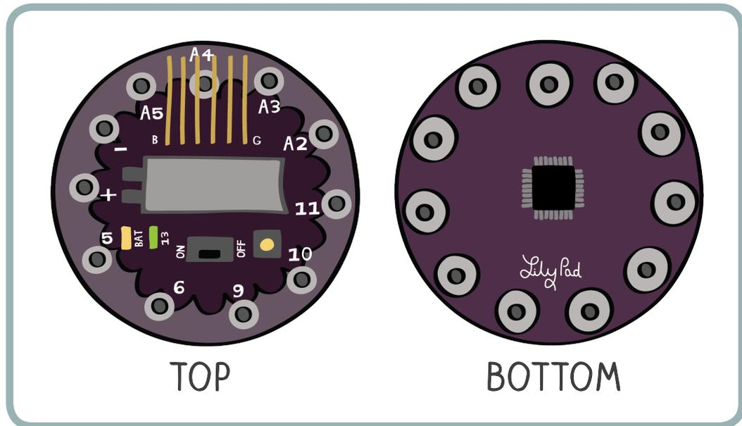
The bottom side of the LilyPad has a ring of snaps surrounding an assortment of electronics. Each snap is connected to one of the tabs on the top side of the LilyPad. The black square in the center of the board is a computer chip called a **microcontroller**. This tiny chip stores programs and controls the electronics that are connected to the LilyPad. Notice that the chip has tiny silver legs coming out of each of its sides. These legs are called **pins**.
