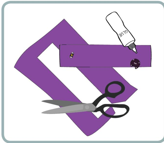
While you are waiting for the glue to dry, use a piece of chalk, a pencil, or a pen to lightly mark on your fabric the traces that go from the battery holder to the LED. This will make it easier for you to sew your connections when you start stitching.
