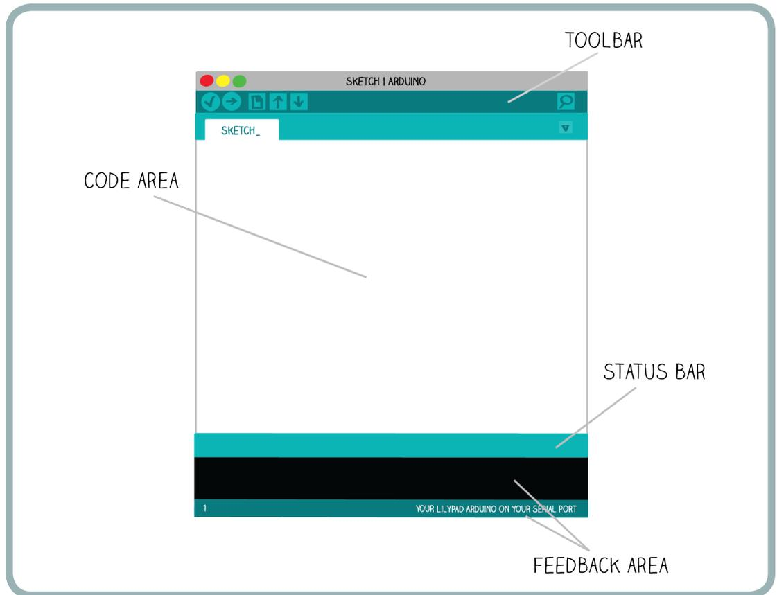
1. **TOOLBAR.** The Toolbar provides you with a quick way to perform common tasks. Each icon in the Toolbar corresponds to a different action.
