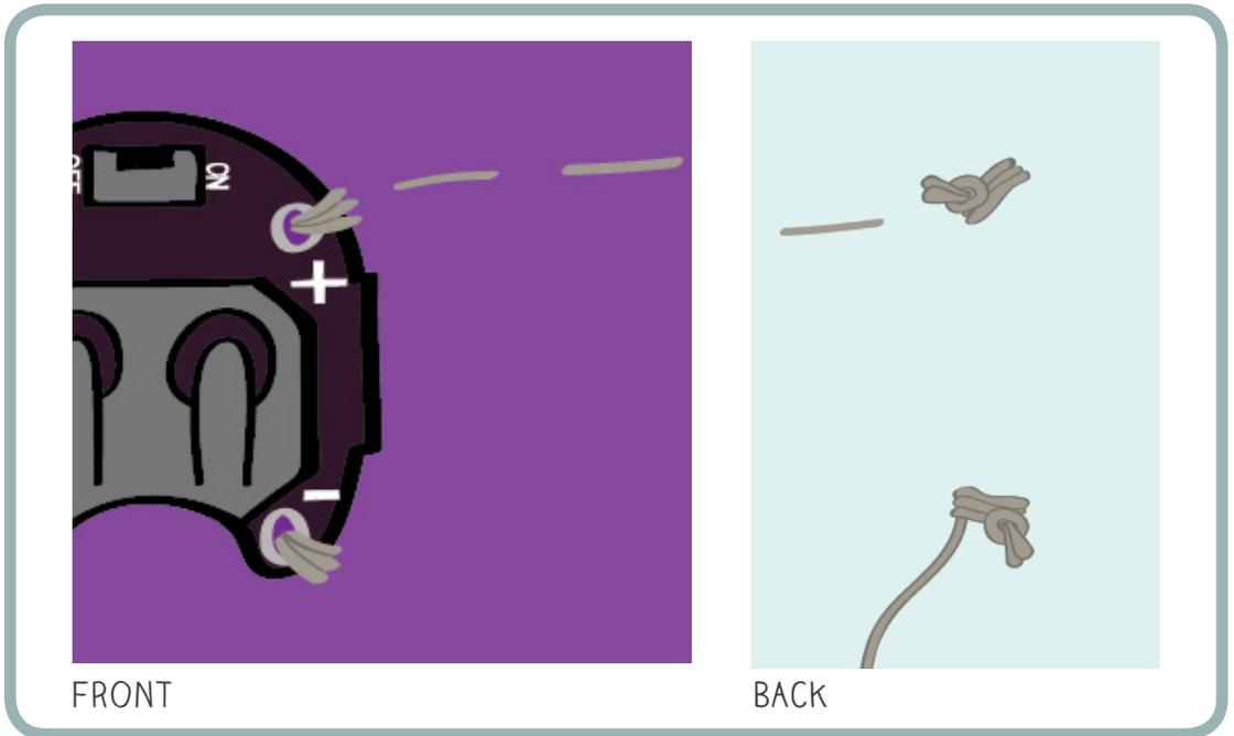
Then, following the line you drew on your fabric, stitch from this tab to the (-) tab on the LED, checking periodically for tangles, loose threads, and puckering. When you reach the (-) tab on the LED, loop through it snugly at least three times before tying a knot, cutting your thread, and securing your knot with a dollop of glue.
