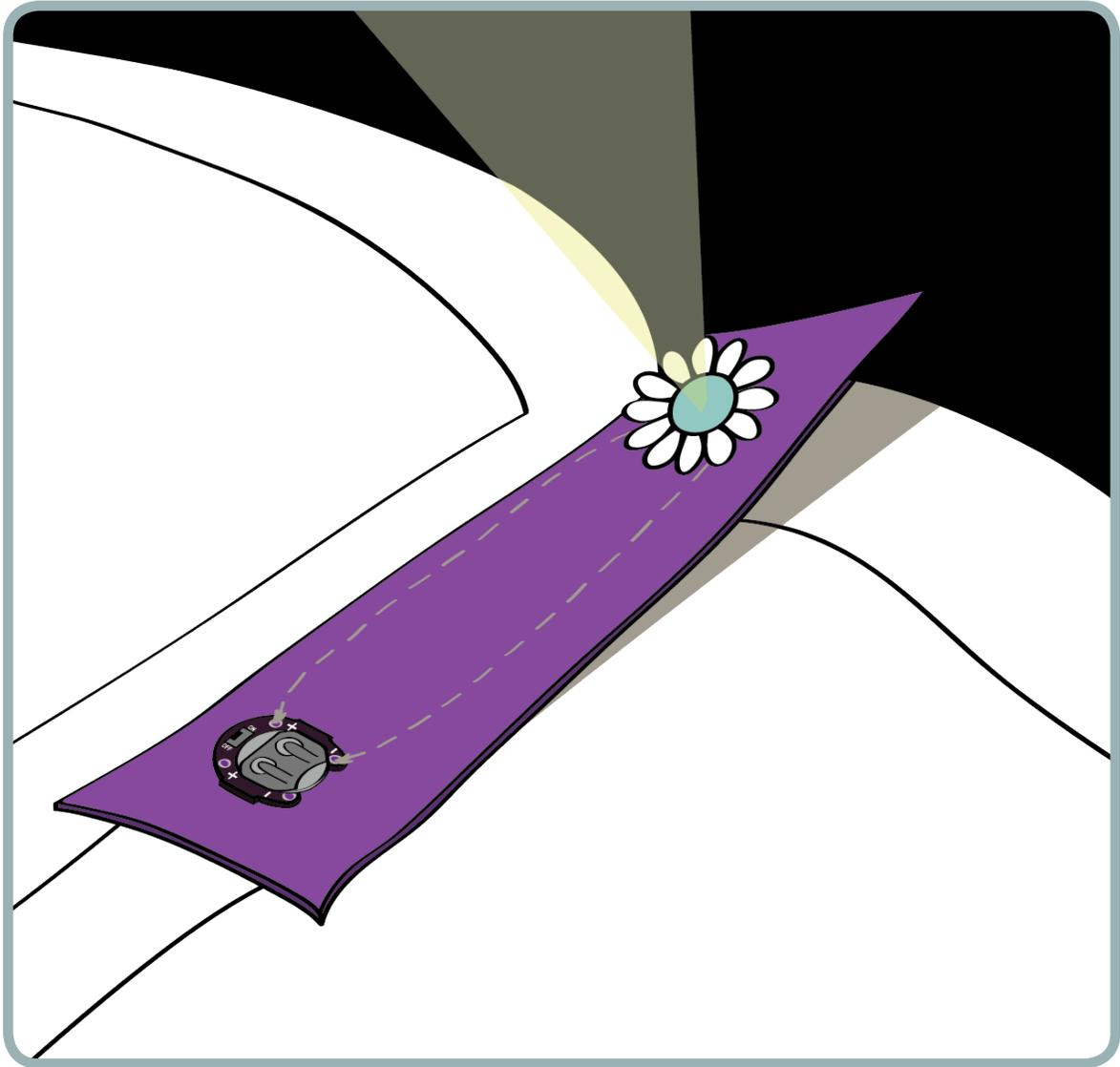
Welcome to the world of electronics and textiles! In this tutorial, you'll explore how to make soft electronic circuits using conductive thread, LEDs, batteries, and fabric. You'll stitch together a fuzzy bookmark that you can use to read in the dark.
