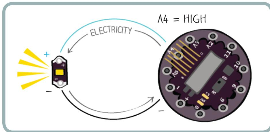
When you set the led pin (A4) LOW with the statement `digitalWrite(led, LOW);`, pin A4 gets set to (-). Since electricity does not flow from (-) to (-), the flow of electricity stops:
