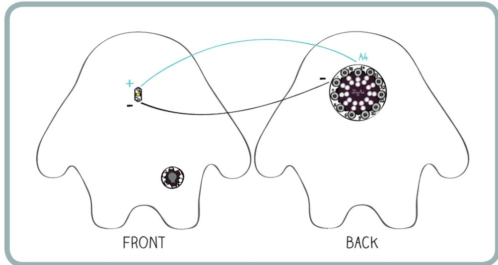
Next, plan the speaker connections. The (-) tab on the speaker needs to be attached to the (-) tab on the LED (shown in black, below). The (+) tab on the speaker should be attached to another tab on the protoboard. Any tab except (-) or (+) will do. Here, the green trace shows the (+) tab of the speaker attached to pin 5.
