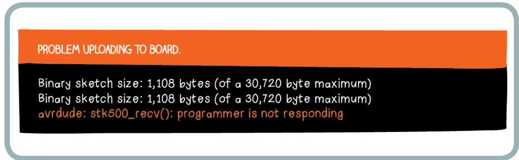
This means that the LilyPad Arduino board is not responding to your computer’s attempts to communicate with it. Possible causes of this error are:
