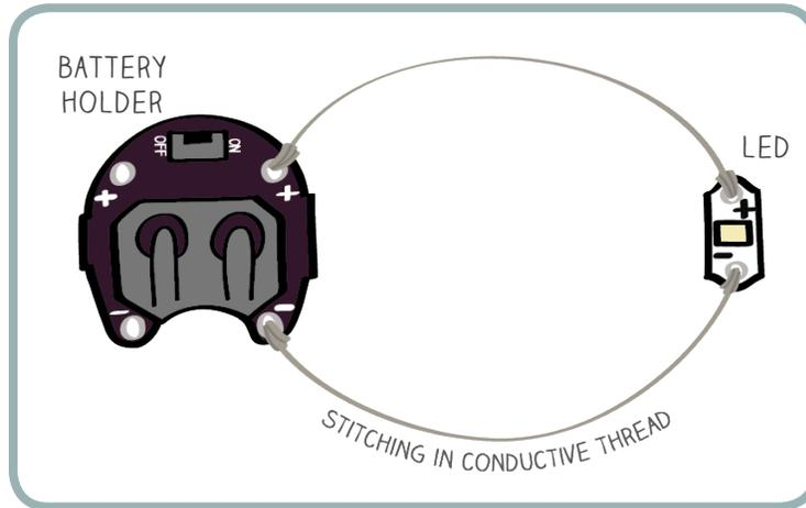
The LED will glow when electricity flows from the (+) side of the battery through the conductive thread, through the LED, and back to the (-) side of the battery.
