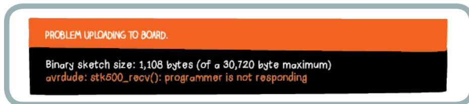
If you receive an error like this, return to the Setup section of this tutorial and make sure that you have completed all the necessary setup steps, including selecting the appropriate Serial Port and board in the Arduino software. If you are still having problems, look through the troubleshooting section of the Arduino website: <http://arduino.cc/en/Guide/Troubleshooting>.
