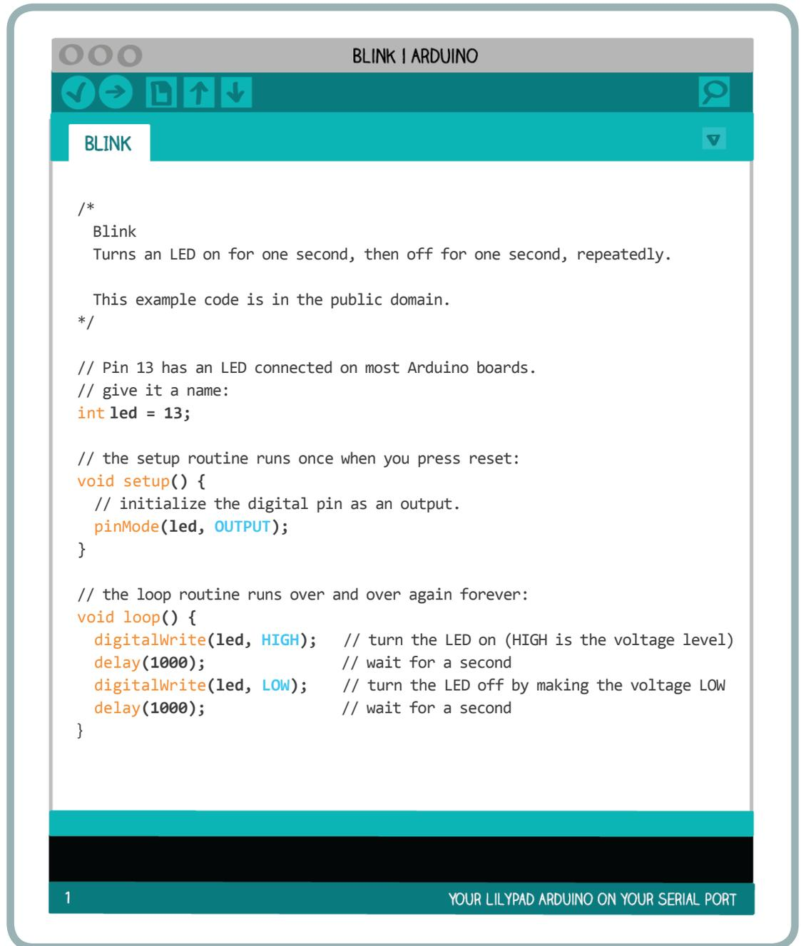
A screenshot of the Arduino IDE interface. The title bar reads "BLINK | ARDUINO". Below the title bar is a toolbar with icons for checkmark, play, save, up, and down. A teal header bar contains the word "BLINK" and a dropdown arrow. The main area displays C code for a blink program. At the bottom, a status bar shows "1" on the left and "YOUR LILYPAD ARDUINO ON YOUR SERIAL PORT" on the right.
