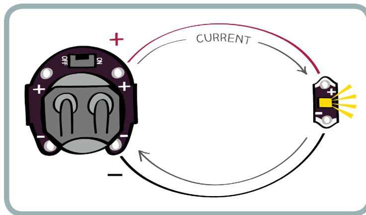
All batteries have two important ratings. They have a **voltage** rating and an **amp-hour** rating. The voltage rating tells you how many volts your battery can supply, and the amp-hour rating tells you how much current it can supply. Together, these two ratings tell you how much **energy** is stored in the battery.
