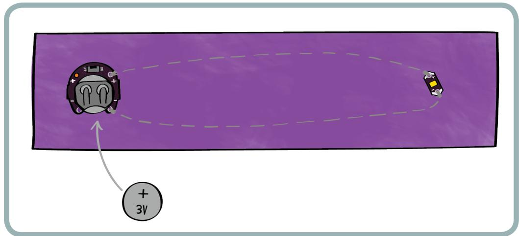
Flip the switch on your battery holder from "off" to "on" to test out your LED. Your LED should now shine brightly. If it doesn't, see the troubleshooting section.
