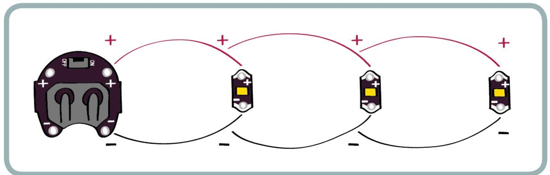
Note that in each of these diagrams, all the (+) tabs on the LEDs are sewn together and all the (-) tabs are sewn together.
