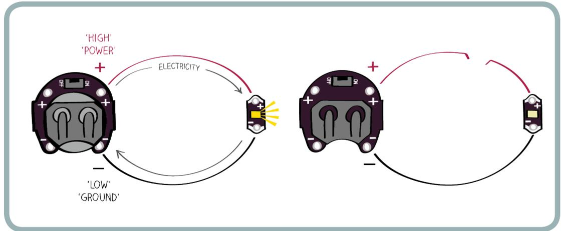
This is how **switches** work. A switch opens up a break in a circuit and then closes it. When you flip a light switch on your wall, this is what it's doing. This is also what is happening when you flip the switch on your battery holder.
