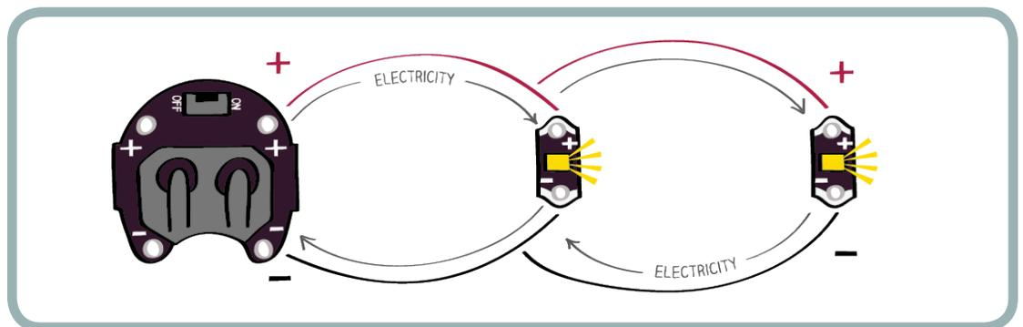
To add an LED to your project, stitch the (+) tab of the new LED to the (+) trace of the original circuit and the (-) tab of the new LED to the (-) trace of the original circuit.
