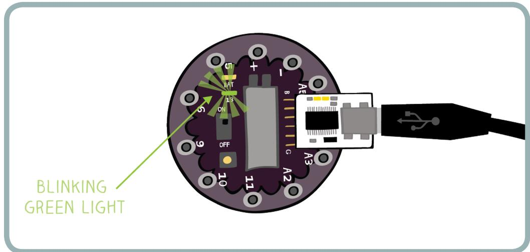
Try unplugging the LilyPad from your FTDI board. Flip the on/off switch on the LilyPad to off. The LilyPad should stop blinking. Now, flip the on/off switch on. The LilyPad should begin flashing again.
