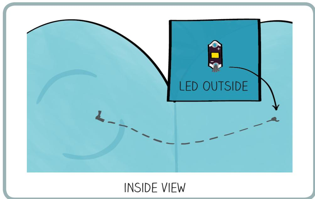
Now sew the (+) side of your LED to the correct pin on the protoboard (A4, or the pin that you chose). Here's an inside view of the monster with both the (+) and (-) LED connections stitched in:
