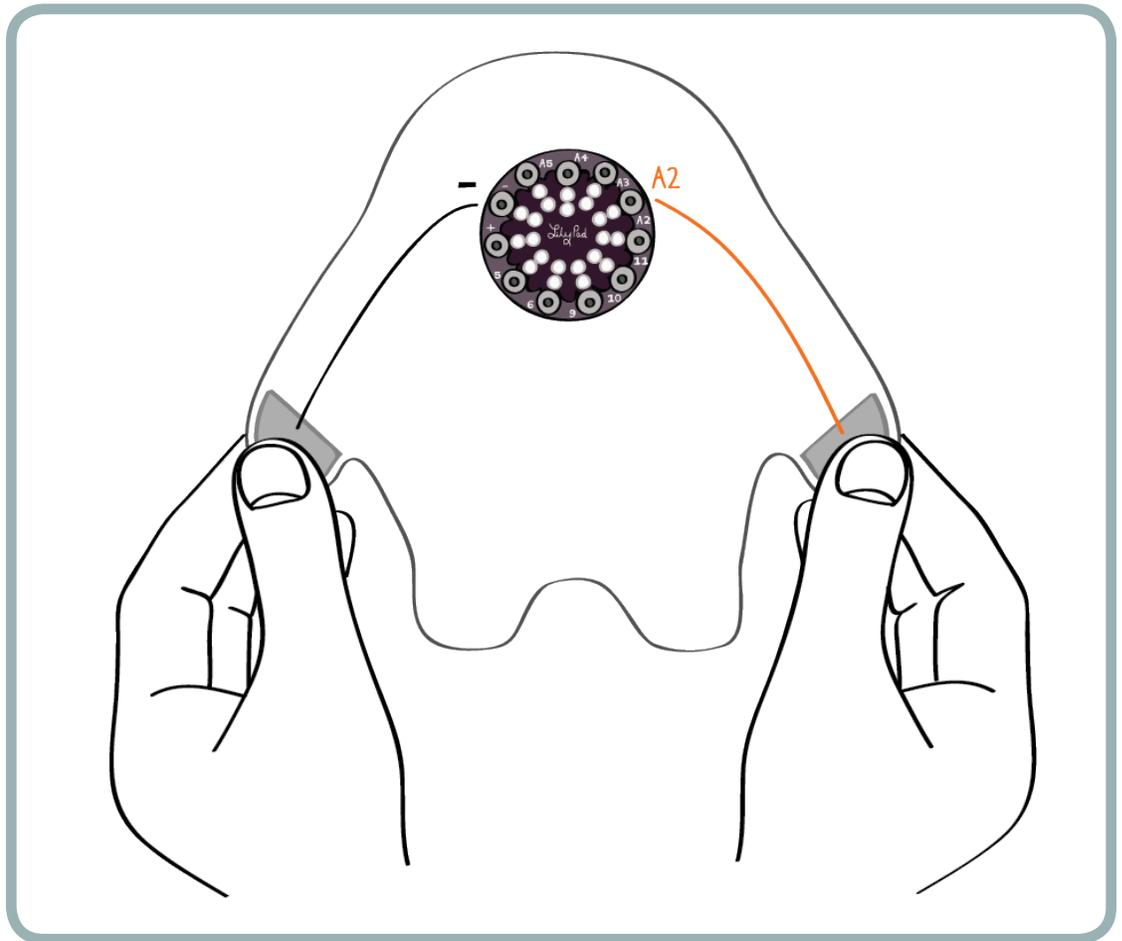
This is why the numbers in the serial monitor go down when you touch the sensor. The harder you squeeze on the sensor, the stronger the connection is between your body and the aluminum foil, and the better the electrical connection is between (-) and A2. This is why you see lower numbers as you squeeze harder. This is also why you see very low numbers (close to 0) when you touch the two paws directly together.
