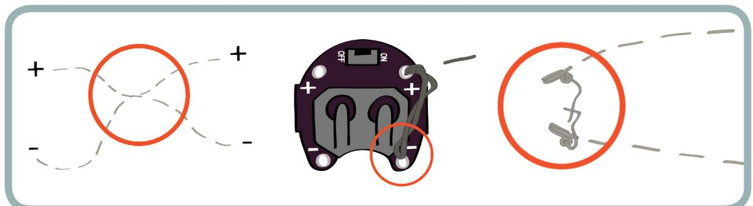
2. Did you use two pieces of thread in this project, or did you sew all the way from (+) to (-), across the LED, with one piece of thread? If you used only one piece of thread, you created a short circuit.
