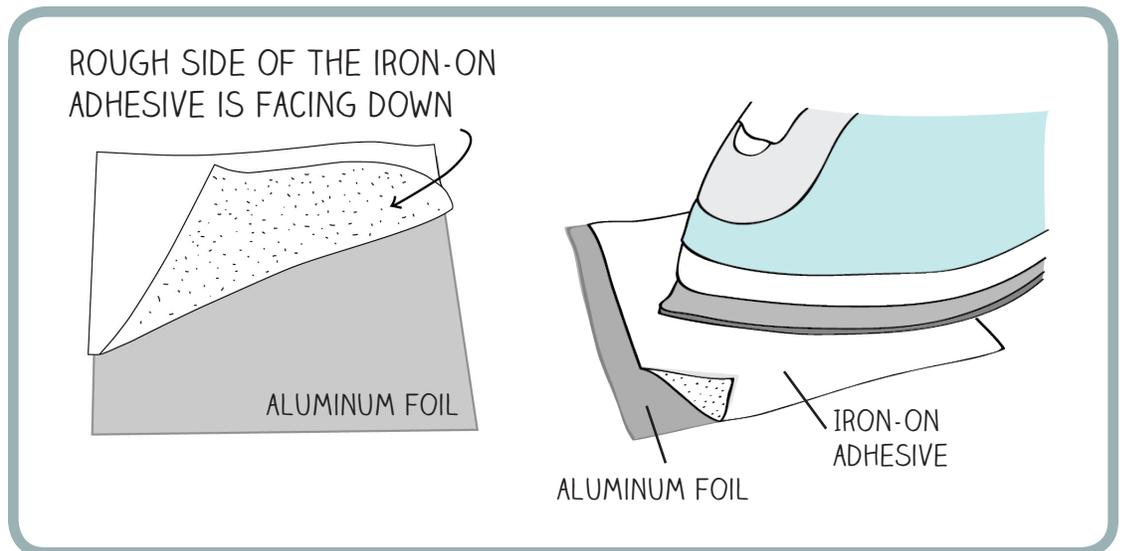
To make sure that the adhesive is firmly attached, peel up a small corner of the paper. It should peel away easily, and you should see a layer of clear adhesive stuck to the aluminum foil. Only peel up enough paper to check on the adhesive. Don't peel away the paper yet.
