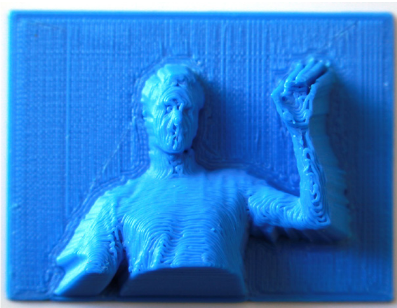
Figure 5-25. Here's the final result of the print from my scan in closeup. You can see the topographical texture left from how the extruder moved around during the course of the print.
