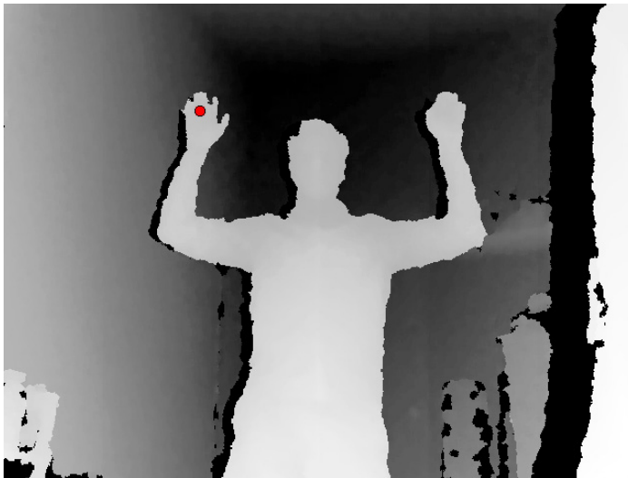
Figure 4-6. The red dot shows up immediately after the completion of calibration, and our sketch begins receiving joint data. Having been converted from real-world to projective coordinates, the joint position vector matches up with the position of the user's hand in the depth image.
