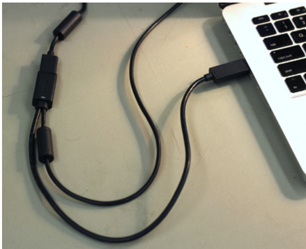
Figure 2-6. The male USB connector from the power supply plugs into your computer's USB port. With the Kinect plugged into the Xbox plug and the power plug in a socket, this completes the physical setup for the Kinect.
