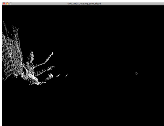
Figure 3-5. The point cloud viewed from the side. The Kinect is directly in front of me, but we're viewing the point cloud from an alternate point of view.
