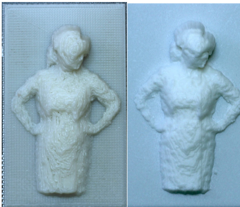
Figure 5-29. Another comparison of a MakerBot print (left) with a Shapeways print (right).
