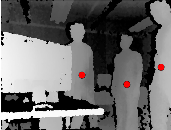
Figure 4-26. Tracking multiple simultaneous users without calibration by their center of mass. This technique is especially effective for installations and projects in public space.
