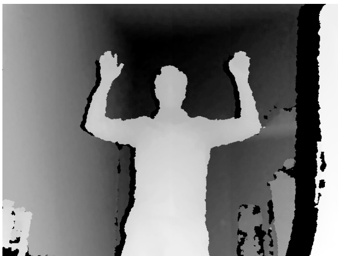
Figure 4-4. This screen capture was taken from within the onEndCalibration callback. I'm clearly holding the calibration pose.
