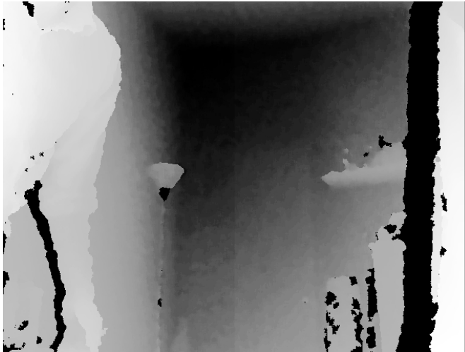
Figure 4-2. OpenNI can tell that a user is in the scene very early. This screen capture was taken from within the onNewUser callback, and you can see I've barely entered the frame on the left.
