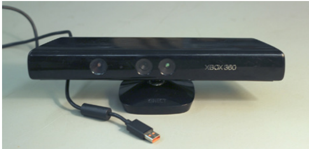
Figure 2-5. The Kinect has one wire coming off of it with a male Xbox connector at the end. This plugs into the female Xbox connector attached to the power plug.
