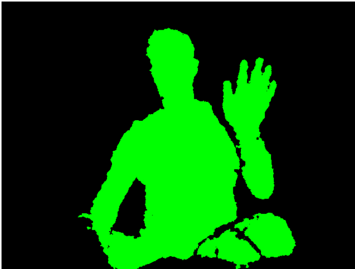
Figure 4-21. Separating the user pixels from the background pixels using getUsersPixels .
