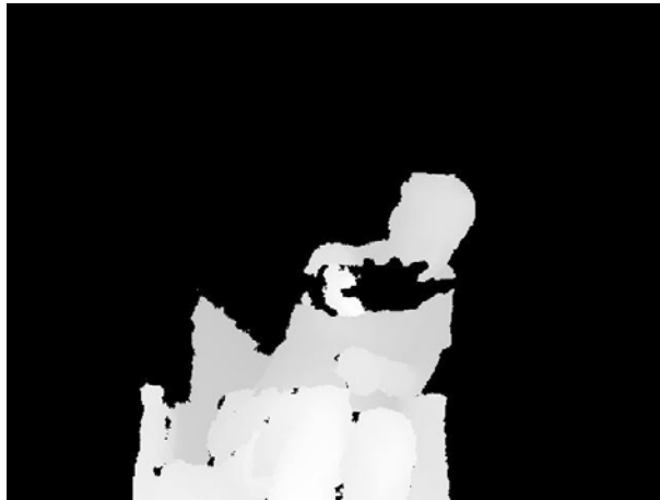
Figure 2-19. The depth image with its range limited to only show the part of the scene that's likely to include the user.
