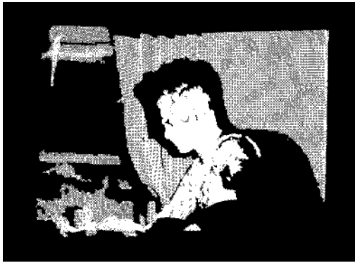
Figure 5-11. Processing displaying the point cloud at the moment we create a mesh.
