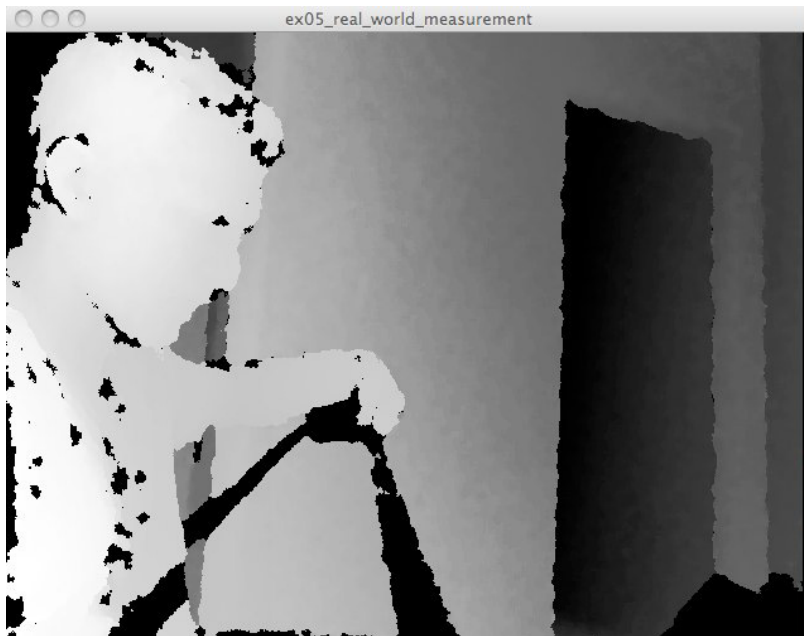
Figure 2-13. I held up a tape measure in front of my Kinect to check our depth measurements against the real world.
