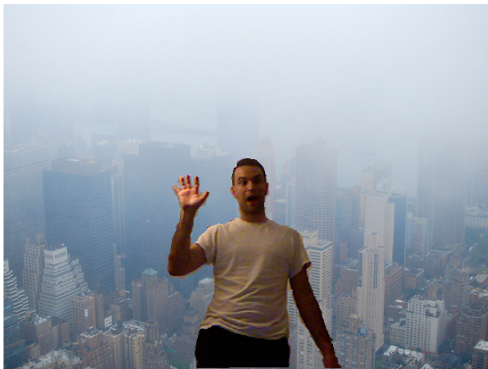
Figure 4-22. Background removal using getUsersPixels . Using OpenNI's user tracking to extract the pixels representing the user from the background. Here I replaced the background with a picture I took from the top of the Empire State Building on a cloudy day.
