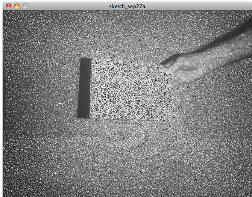
Figure 1-2. An image of the normally invisible grid of dots from the Kinect's infrared projector. Taken with the Kinect's IR camera.
