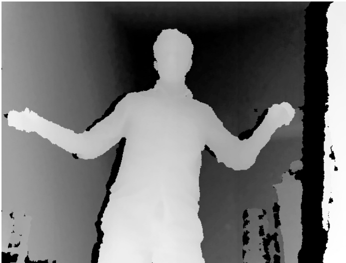
Figure 4-3. This screen capture was taken from within the onStartPose callback. OpenNI can tell that I'm in the start pose even though I don't have my arms fully in position.
