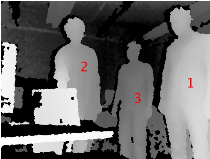
Figure 4-27. We can distinguish individual users in our scene as they move across each other in the space and even keep track of them if they briefly leave the frame and then return.
