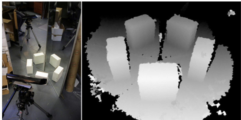
Figure 2-10. Artist Kyle McDonald's setup using mirrors to turn the Kinect into a 360 degree 3D scanner. Photos courtesy of Kyle McDonald.
