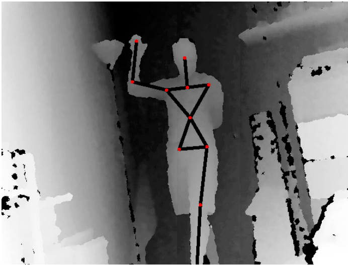
Figure 4-11. If the confidence score is too low for the given joints, SimpleOpenNI 's drawLimb function will hide the affected limbs—in this case, my left upper and lower arm and my right thigh and shin.
